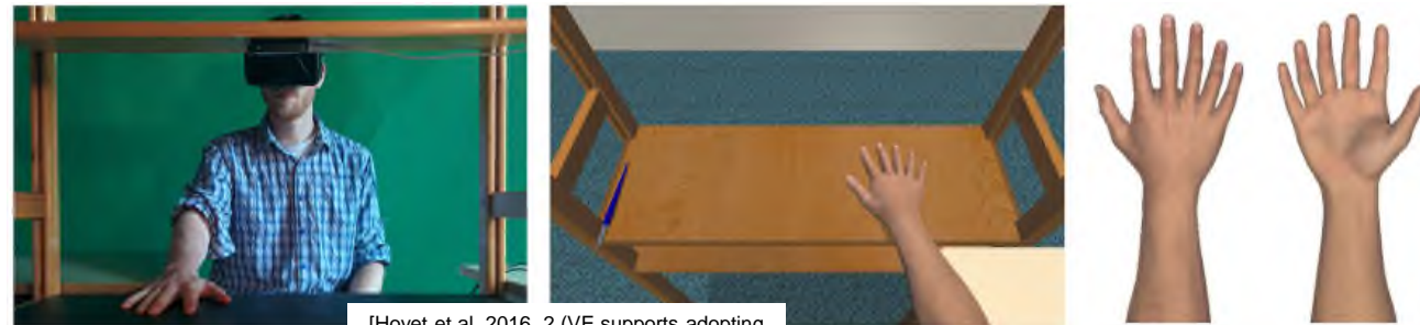
FIGURE 1 | Setup of the experiment. Left: physical experimental setup. Middle: corresponding virtual setup including the six-digit virtual hand used in the experiment. Right: six-digit virtual hand model used in the experiment.
